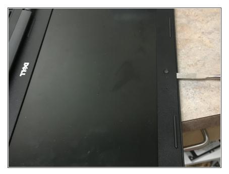
Using a spluger pry the bezel from the back cover. Be careful there is tape and clips holding this bezel on but its not too back to remove.
