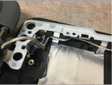
Remove this wire from the back cover. You will need to either pry up or cut the foil tape. Also remove the screw that hold the tiny board up near the top of the back cover.
