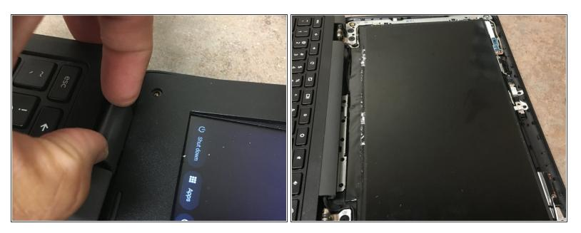
To finish removing the bezel allow the prying of the bezel to pop loose the hinge covers then remove them for easier access to the wires.
