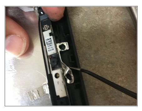
Remove the camera board from the back cover. It has foil take attaching it to the cover so carefully pry that off.
