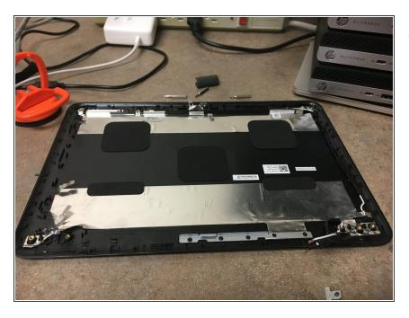
This LCD back lid comes with the metal tape and wifi wire already attached. This guild is based on purchasing this model WITHOUT the camera board. You can buy them with the camera board if you wish.
