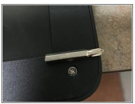
Remove the dot screw covers from the 4 corner screws of the bezel.
