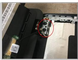
Remove the hinge/lid brackets. To do this remove the 4 black (LARGE HEAD) scres
