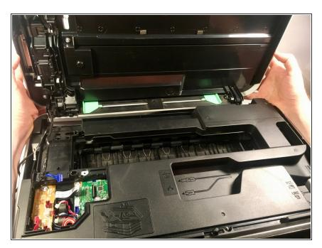
Using both hands, pull the scanner cover to the rear while holding it vertically, then lift it off of the printer.
