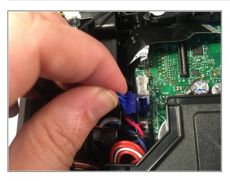
Pull the ADF motor harness out of its socket.
