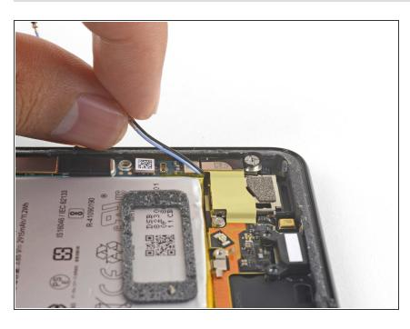
Carefully de-route both antenna cables and move them away from the charging assembly.
