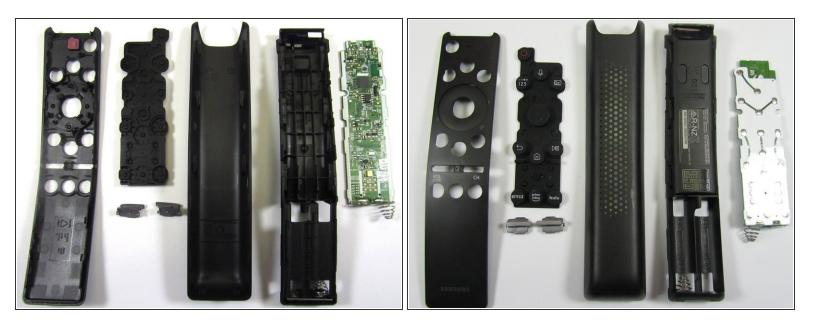
• Teardown Exploded Views of the Frontside and Backside of Samsung QLED TV Remote
