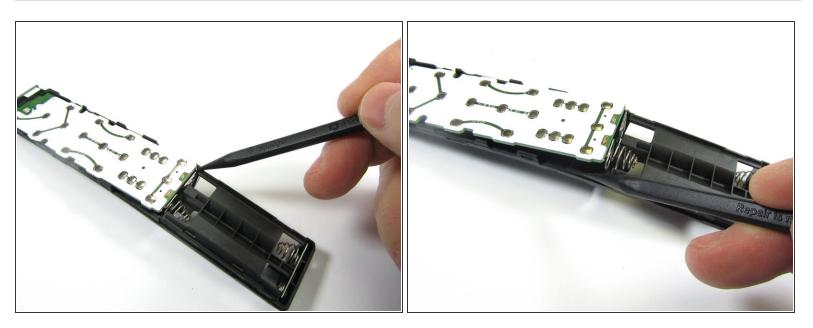
To remove the PCB from the enclosure, use the Spudger Tool to gentle pry up on both sides of the bottom part of the PCB near the battery compartment area. This will release the PCB from the PCB enclosure.
