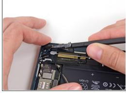
Use the flat end of a spudger to loosen the foam adhesive holding the GPS antenna to the right speaker.
