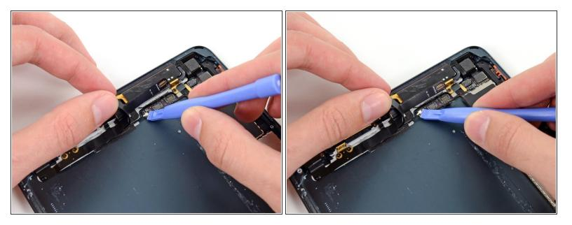
• Use a plastic opening tool to pry the top left antenna cable up from its socket on the logic board.
