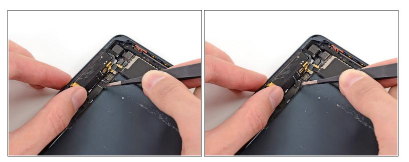
Use tweezers to peel up and remove the small piece of tape covering the headphone jack cable connector.
