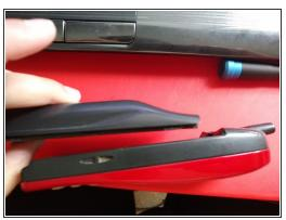
Remove the battery by pushing the button and sliding the battery out a bit then pulling it out
