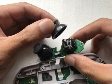
Hold the analog board assembly along the edges, and carefully pull out the old analog stick caps one-by-one.
