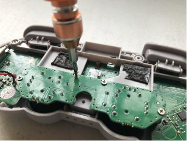
Unscrew the four #0 Phillips screws that hold the analog board in place.
