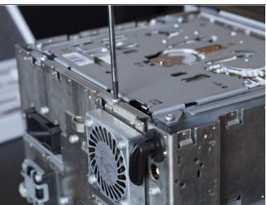
Remove five 6 mm T9 Torx screws from the top side of the unit.
