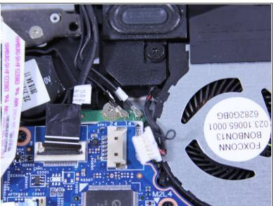
Pull the clipped cables from system board (motherboard).
