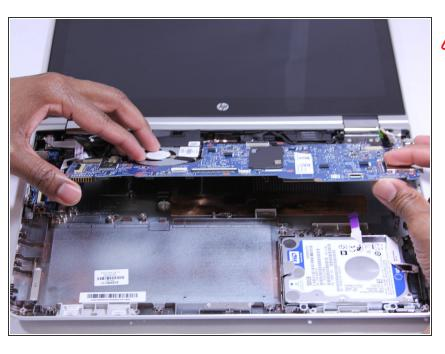
Carefully lift the front side of the system board (motherboard).
