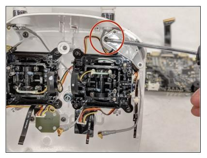
Remove the 10.7 mm Phillips screws using a Phillips #1 screwdriver.
