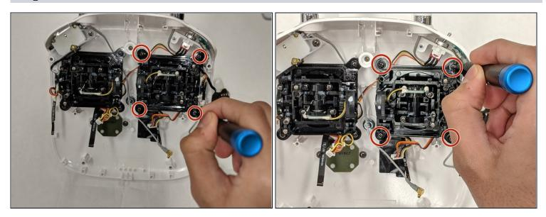
• Remove the 4 10.7 mm Phillips screws using a Phillips #1 screwdriver.
