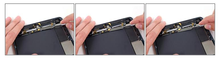
• Slowly work the flat end of a metal spudger underneath the microphone cable, separating the adhesive securing it to the headphone cable.
