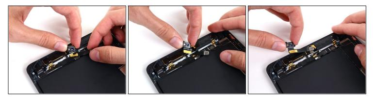
• Carefully remove the front-facing camera from the iPad, threading its cable through the slot cut near the bottom of its socket in the rear case.
