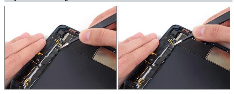
• Use a pair of <u>tweezers</u> to peel up and remove the small piece of tape covering the front-facing camera cable connector.
