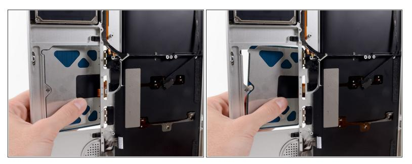
With the cable free, remove the trackpad from the upper case.
