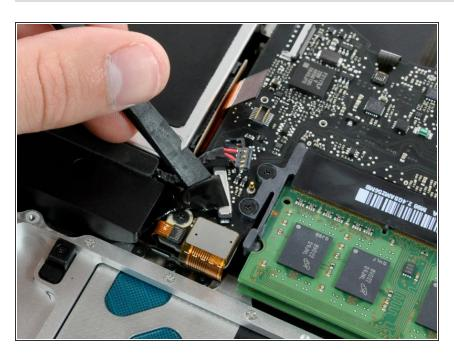
Use the flat end of a spudger to pry the silver-colored hard drive cable connector straight up out of its socket on the logic board.
