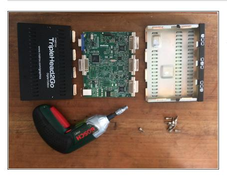
To reassemble the card, just go the same way back. You can see the positions of the copper pieces in the previous step (I guessed them by the marks in the metal), and the one of the screws in the first step. Easy, isn't it?
