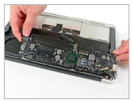
Gently lift the logic board assembly out of the upper case, minding the fragile heat sink and any cables that may get caught.
