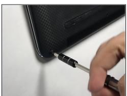
Using a T5 Torx screwdriver, remove ten 3mm screws.
