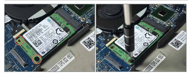
Using a Phillips #0 screwdriver, remove two 2.5mm screws that secure the SSD to the chassis.
