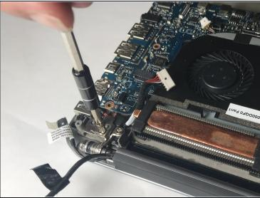
• Using a Phillips #0 screwdriver, remove the four 4mm screws holding in the screen hinges.
