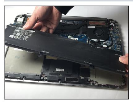
• Lift the battery off the chassis.
