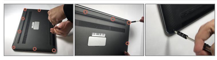
Using a T5 Torx screwdriver, remove ten 3mm screws.
