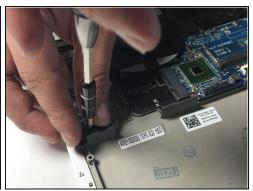
• Remove the three 3.5mm Phillips #0 screws mounting the motherboard.
