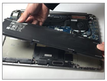
• Lift the battery off the chassis.
