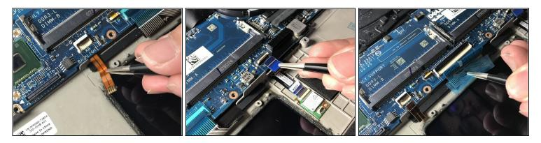
• Disconnect ribbon cables above the touch pad using <u>tweezers</u>.
