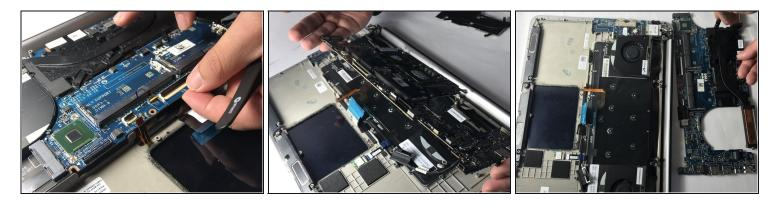
Lift and remove the motherboard from the chassis.
