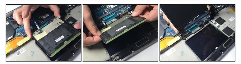
Lift the bottom of the touchpad and pull directly out.
