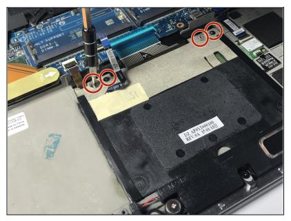
Using a Phillips #0 screwdriver, remove the four 3mm screws holding in the touchpad assembly.
