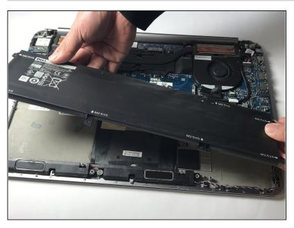
• Lift the battery off the chassis.
