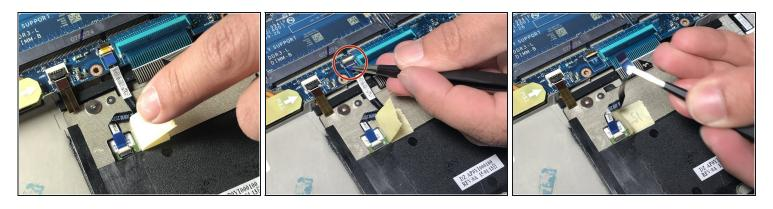
• Remove the touch pad ribbon cable by lifting the small plastic flap and pulling ribbon straight out of the connector.
