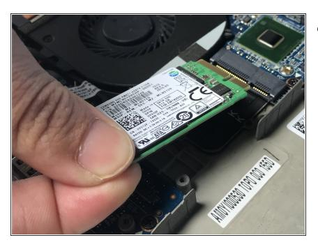
Pull the SSD out parallel to the mainboard.
