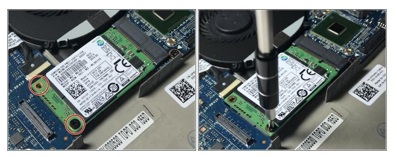
Using a Phillips #0 screwdriver, remove two 2.5mm screws that secure the SSD to the chassis.
