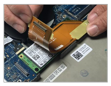
Pull lift tabs and remove the plastic that covers the hard drive to expose the hard drive.
