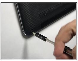
Using a T5 Torx screwdriver, remove ten 3mm screws.
