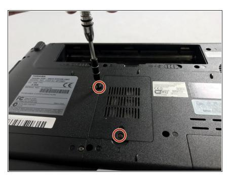
Remove the two 3mm Phillips #00 screws holding the plastic cover over the RAM modules.
