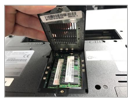
Gently lift the plastic cover. Once the plastic cover is removed, the two RAM cards will be visible.
