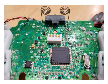
Remove two screws from the D-Pad using a Phillips #0 Screwdriver, After doing so, you will see two latches underneath the screws that you just removed and you have to press the two latches at the same time to completely remove the D-Pad.
