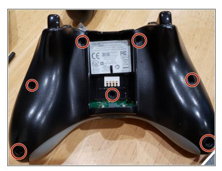
Remove 7 screws located on the back of the controller using the TR-9 Toolbit
