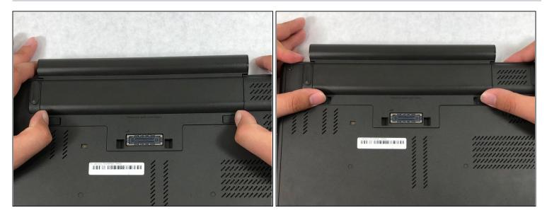
• Slide the battery latches to the unlocked position.
