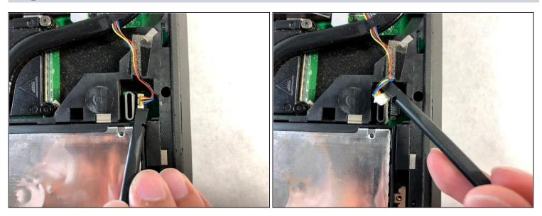
• Using the spudger detach the cable that is connected to the computer.
