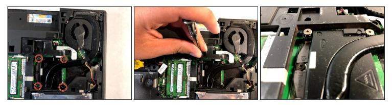
⚠ Screws are attached to the heat sink. Do not try to remove them; just have the screws loosened.
