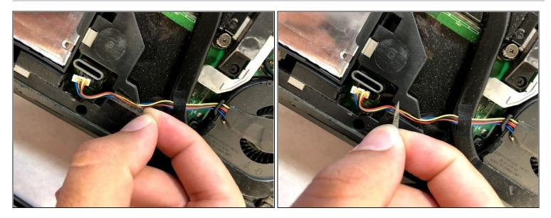
• Remove the tape that is over the cable.
