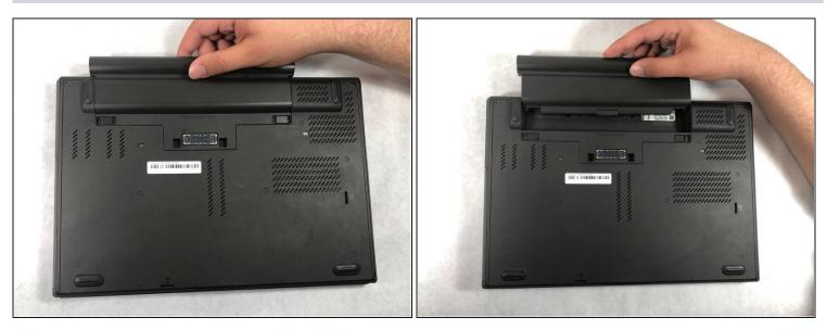
• Slide the battery pack out of the battery slot.
