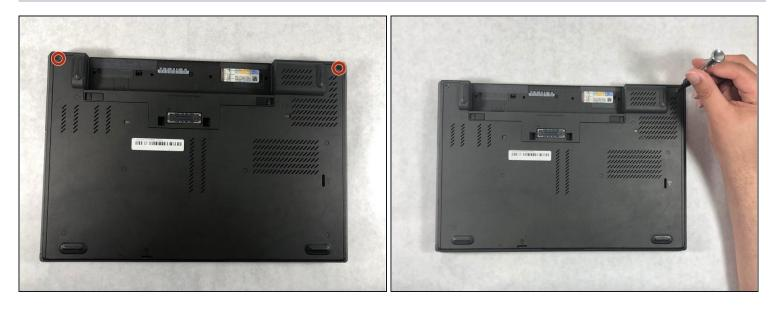
• Use a Phillips #1 screwdriver to remove the two 9mm screws holding the back cover.
