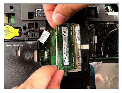
• Remove the RAM by holding on its edges.
