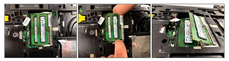
• In the first memory slot, use your fingertips to spread the two white tabs that are holding down the RAM. The RAM will raise to an angle.
