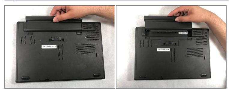
• Slide the battery pack out of the battery slot.
