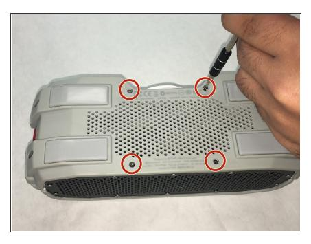
Remove four 1.3 cm inner screws in the outer shell using the 1.5mm Hex screwdriver.
