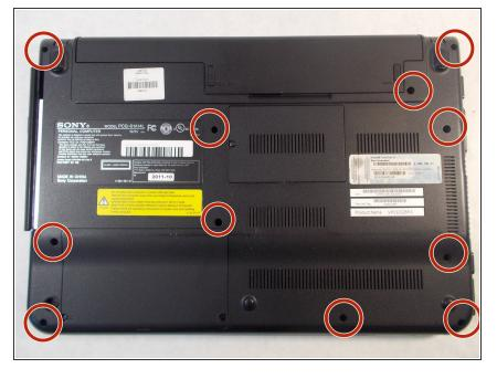
Remove the remaining eleven 7mm screws from back panel using the JIS #0 screwdriver.
