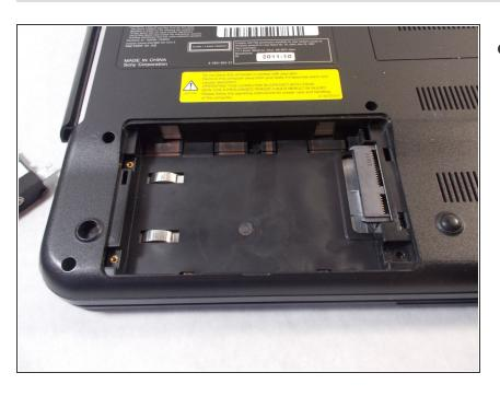
Remove the hard drive from the device.
