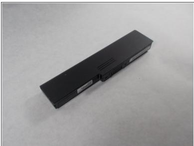
Remove the battery from the battery compartment.
