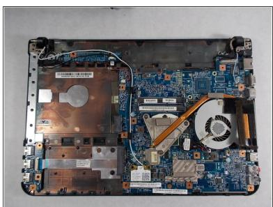
Remove the back panel from the device.
