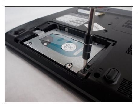
Remove the plastic and unscrew the screw on the hard drive using the JIS #0 screwdriver.
