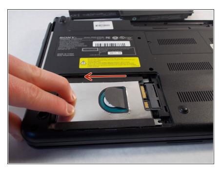
Push the hard drive towards the optical reader to unlock it.
