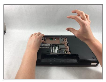
Gently pull the hard drive to the right away from the connector. When fully disconnected you have safely removed the hard drive!
