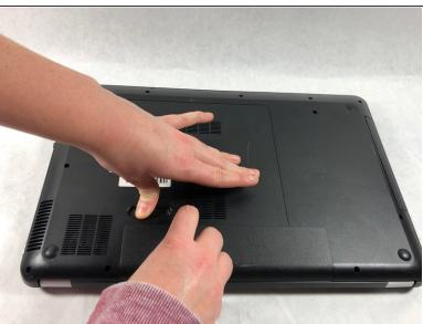
Slide the battery removal switch towards the center of the laptop until the battery pops out.
