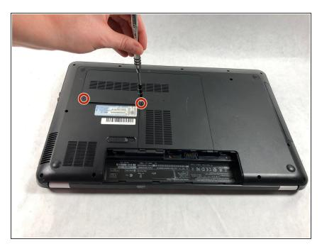
Unscrew the two 4mm Phillips #0 screws found in the surface panel.
