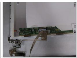
Pull up on and turn over the screen to expose the wire connecting the webcam to the screen.
