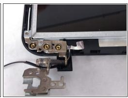
Remove the three 4.1 mm Phillips #0 screws attaching each hinge to the screen.
