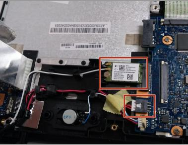
Pull out the wide cable to reveal the components underneath.
