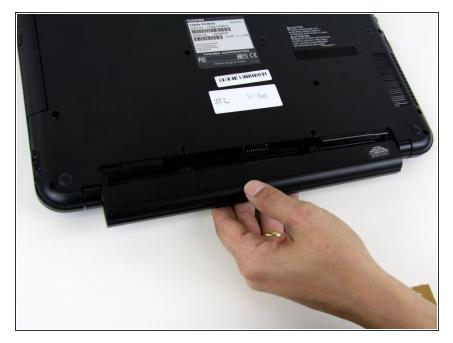
Pull the battery from the back of the laptop for removal from the laptop.
