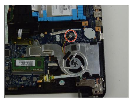
Disconnect the fan wire from the motherboard.
