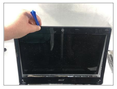
Push the blue opening tool between the edge of the computer and the screen. Slide the tool around the perimeter of the screen.
