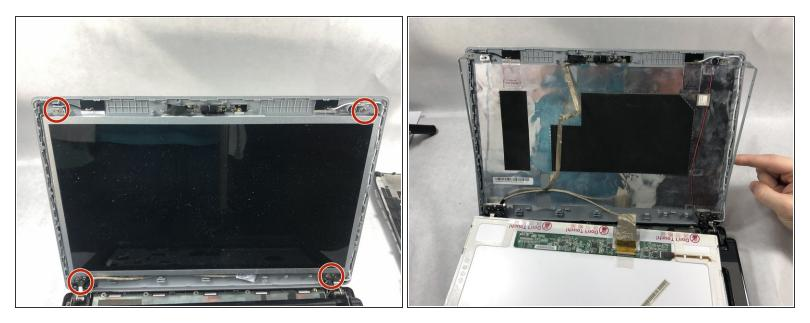
• Remove the six screws from the four corners of the screen using a Phillips #0 screwdriver.
