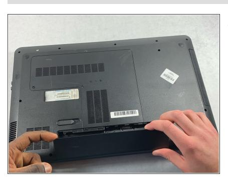
While pushing the switch, lift the battery by the side closest to the switch up and away from the laptop.
