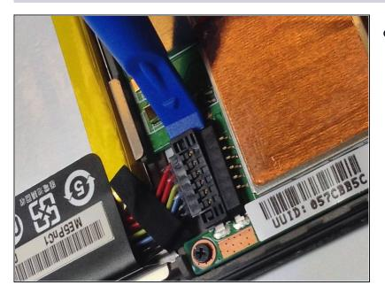
Insert the plastic opening tool under the side edge of the battery connector, and gently pry upward to disconnect it.
