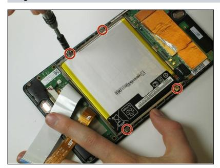
Use the #0 Phillips Screwdriver to remove the four silver 3 mm Philips #0 screws from around the battery housing.
