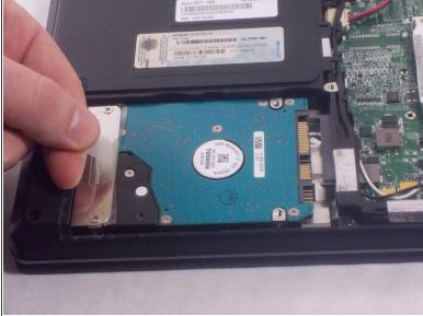
Pull the plastic tab toward the frame to disconnect the hard drive SATA.
