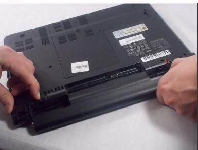
While holding the left tab to the left the battery should easily pull out of the laptop.
