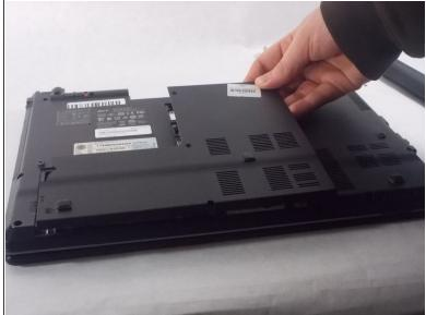
Place laptop bottom side up, and use a Phillips #1 screwdriver to unscrew the five 8 mm screws from the back panel.
