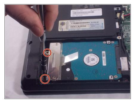
After removing the back panel, use a Phillips #1 screwdriver to unscrew the two 8 mm screws that hold the retaining piece to the frame.
