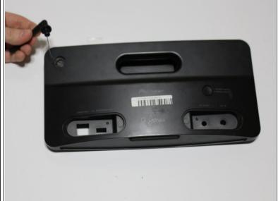
Flip over the back panel and pull the antenna up and out.
