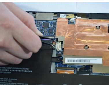
Remove the white connector clip from the connector port using a sturdy tweezers.
