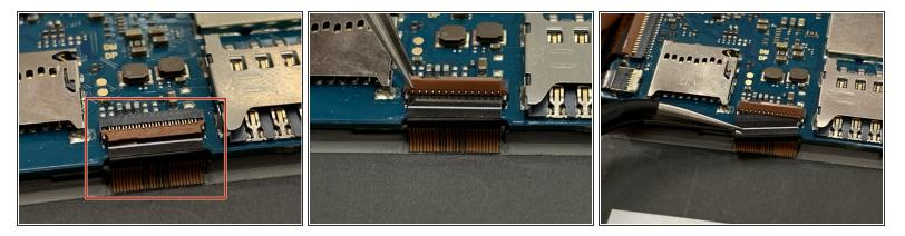
The ribbon cables are attached by zero insertion force (ZIF) connectors. To disconnect the cable, flip up the small locking flap and pull the cable out.
