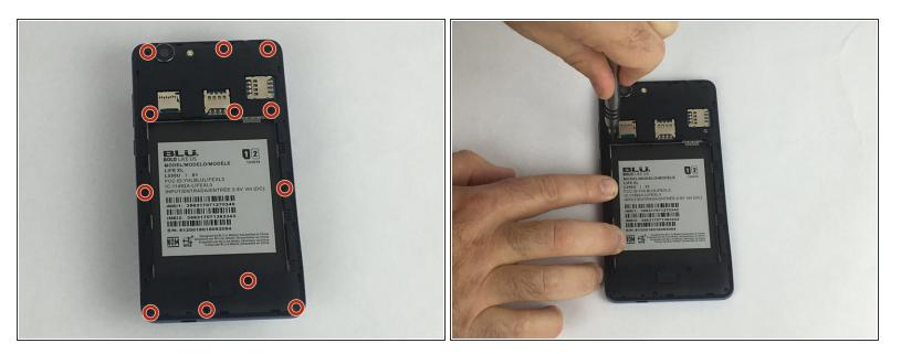
• Remove the 12x3mm screws from the rear plate using the Phillips#000 screwdriver.
