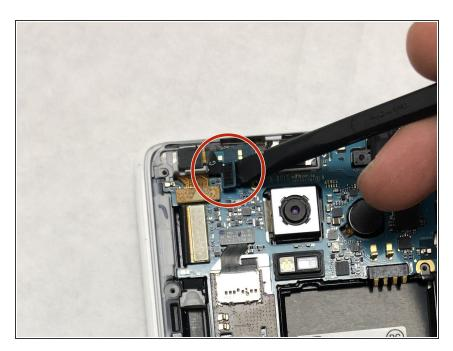
Remove the connection for the front camera.
