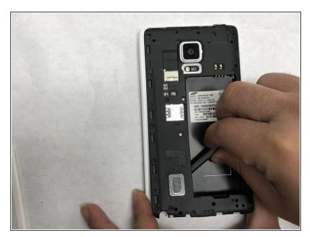
Use a Spudger to remove the black chassis and expose the motherboard.
