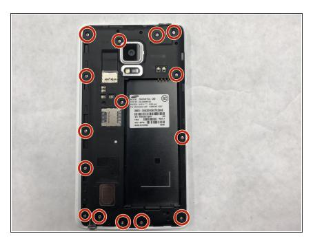
Use a Philips #000 Screwdriver to remove the fifteen 4mm screws.
