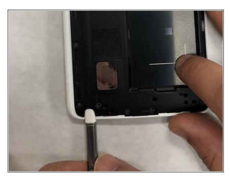
Remove the stylus from its sheathe.
