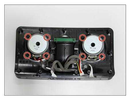
Use a Phillips #1 screwdriver to remove the eight 12 mm screws from the left and right speakers.
