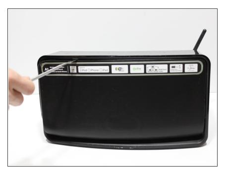
Use the spudger to remove the mesh front panel.
