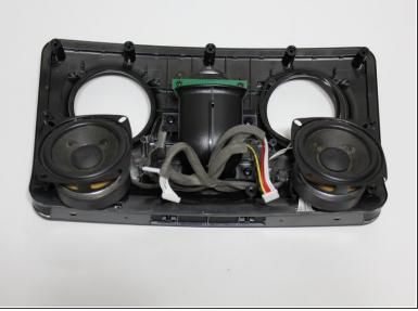
Remove the left and right speakers from the speaker frame by pulling gently up and detaching the wires.
