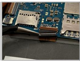
• The ribbon cables are attached by zero insertion force (ZIF) connectors. To disconnect the cable, flip up the small locking flap and pull the cable out.
