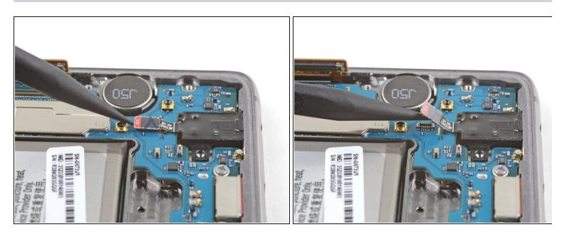
• Use the point of a spudger to pry up and disconnect the headphone jack's connector from its motherboard socket.
