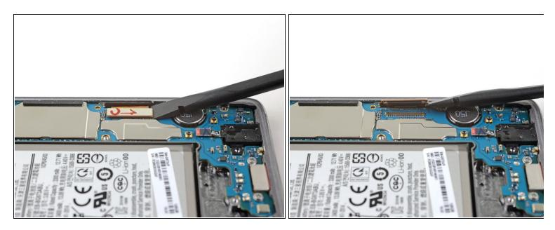
• Use the flat end of a spudger to pry up and disconnect the display connector from its motherboard socket, located near the bottom right corner of the phone.
