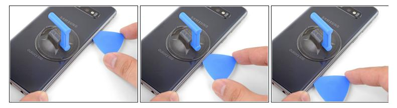
• Slide the opening pick along the edge of the phone, slicing through the adhesive.
