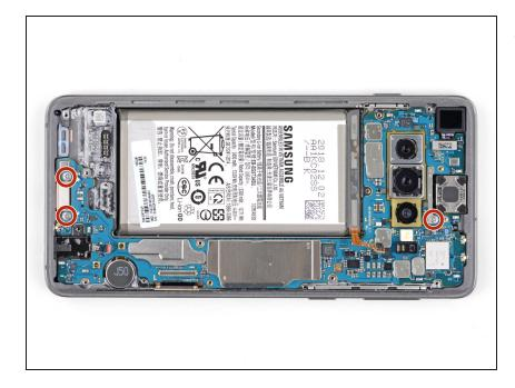
Remove the three 3.7 mm Phillips screws securing the motherboard to the phone.
