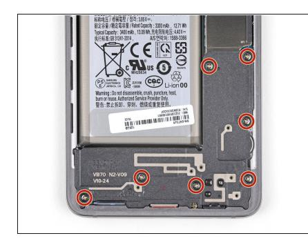
Remove the seven 4 mm Phillips screws securing the lower midframe.
