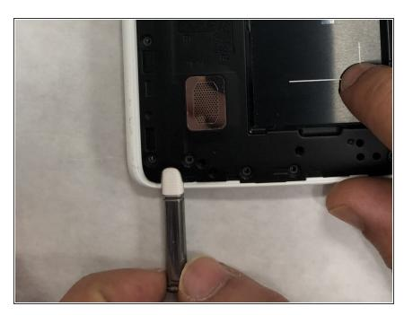
• Remove the stylus from its sheathe.
