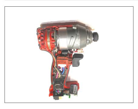
Remove the drill casing to expose the drill's interior parts.
