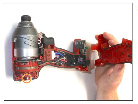
Once the interior is open locate the output shaft driver pictured at the left of the screen.
