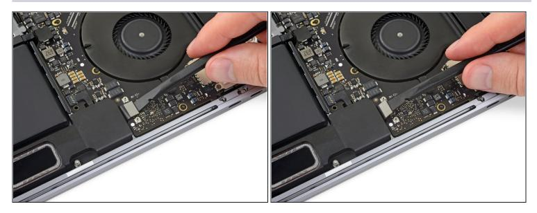
• Disconnect the Touch Bar display cable by prying its connector straight up from the logic board.
