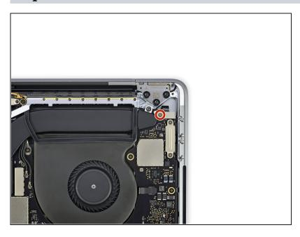
Use a T3 Torx driver to remove the 1.3 mm screw securing the cover bracket for the Touch Bar digitizer connector.
