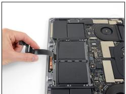
Carefully peel the trackpad cable up off the battery, and push it out of the way.
