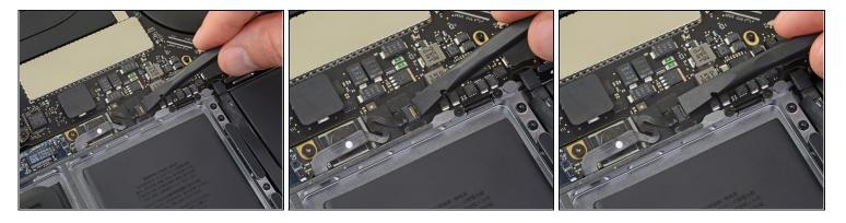
• Use a spudger to gently pry up the locking flap on the <u>ZIF connector</u> for the battery board data cable.
