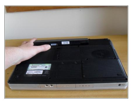
Remove the battery before starting
