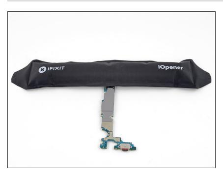
Heat an iOpener and lay it over the rear-facing camera module for one minute. This helps loosen the adhesive holding the camera module to the motherboard.
