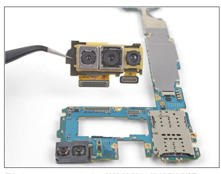
Remove the rear-facing camera module.
