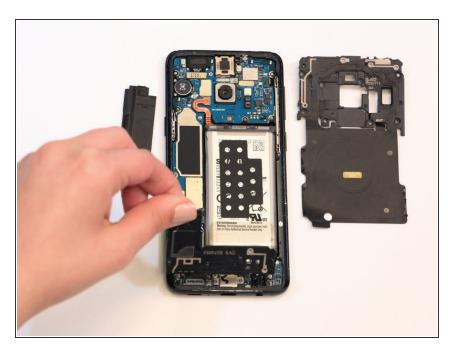
Remove the speaker cover/antenna assembly.
