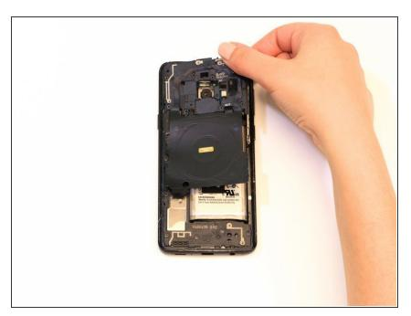
Remove the NFC coil assembly.
