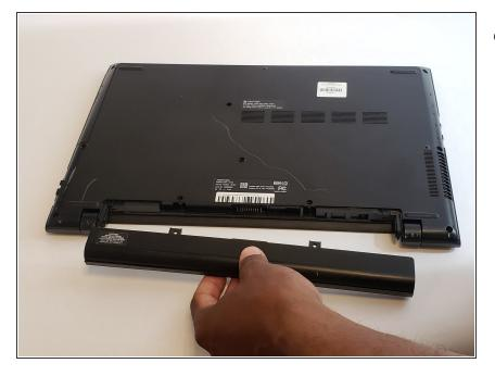
Gently remove the battery in outwards motion. The battery should come out with ease.
