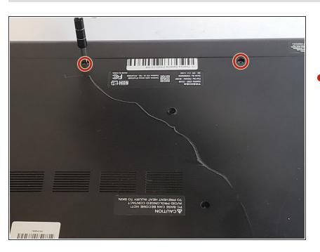
Remove screws on the back of the device securing the battery with a Phillips #1 screwdriver.
