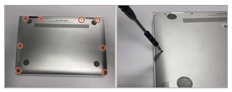
• Using the Torx T5 screwdriver, remove the eight 8 mm screws on the bottom case of the laptop.
