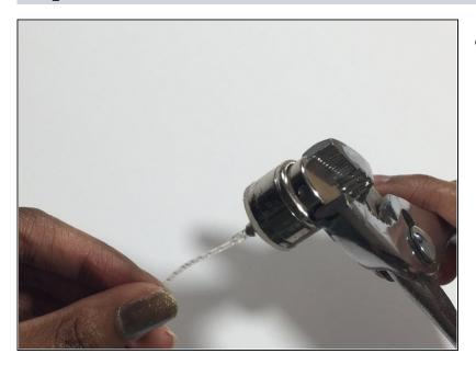
Using the pliers, gently twist the jammed nozzle in a clockwise motion until the pump pops up.
