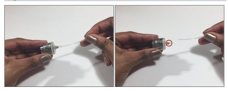
Using your hand, gently pull out the tube so that the metal ball is exposed.
